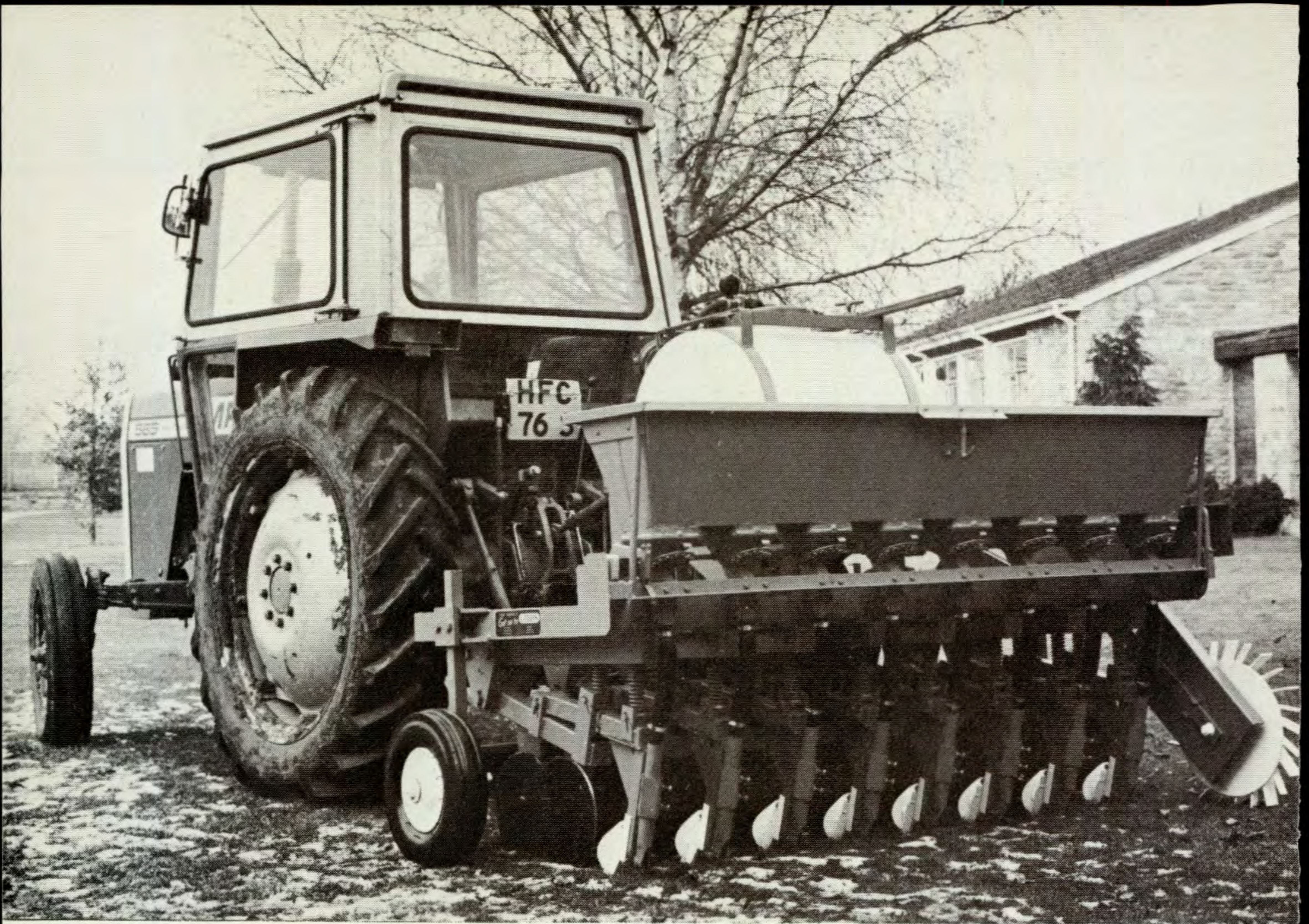
The Gibbs slot seeder; a commercial product built to meet the requirements of the WRO one-pass seeding technique for renovating permanent pasture.
