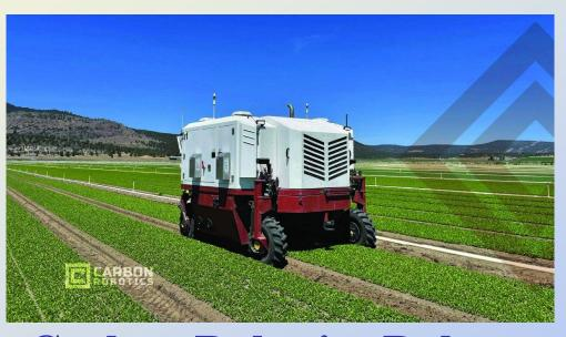
Carbon Robotics Robot - 4.3 tonnes, 73Hp
