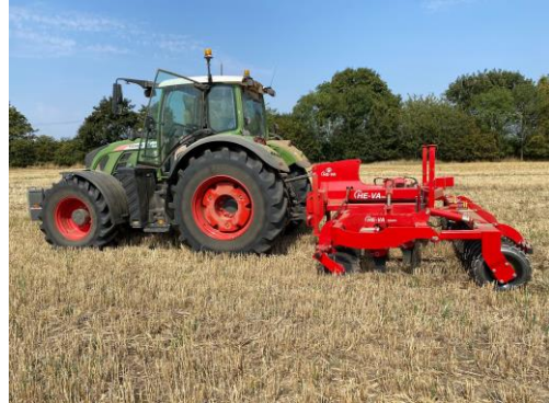
4m He-Va Stealth Low Disturbance Subsoiler
