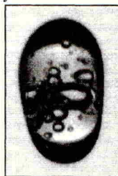
Figure 3. In-flight image of a ca 1 mm diameter water droplet with air inclusions
