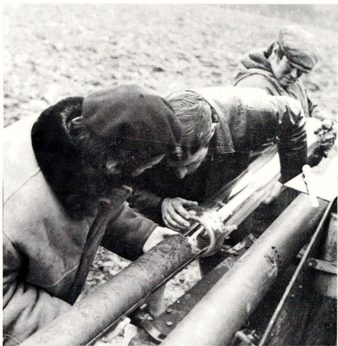
Figure 13. Transfer of cores from sampler to glass columns.
