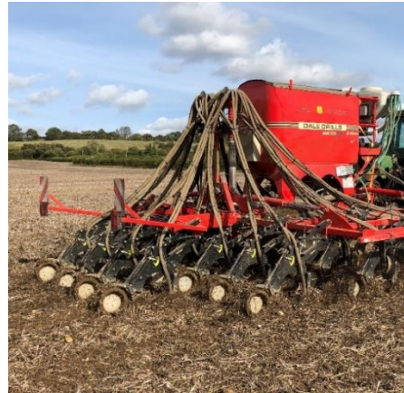
Sustainable System 1: 10-15 cm depth non- inversion cultivation
