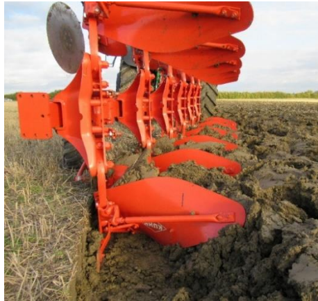
Conventional: 15-20 cm depth inversion cultivation
