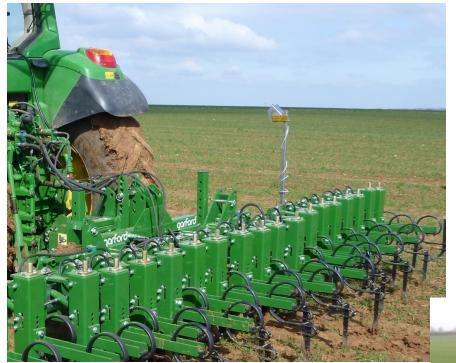
The computer continually adjusts the position of the hoe via a hydraulic sideshift or disc steer system.
