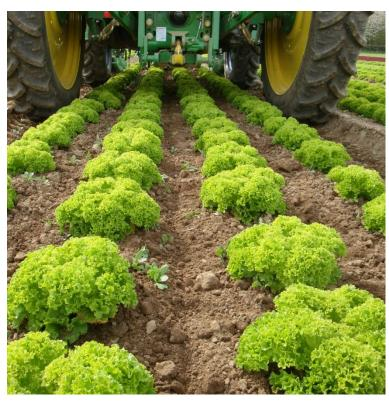
The latest Robocrop Inrow eRotor model can work with high accuracy at up to 6 plants per second per row resulting in spot workrates of more than 3 hectares per hour for this split 6mtr model.
